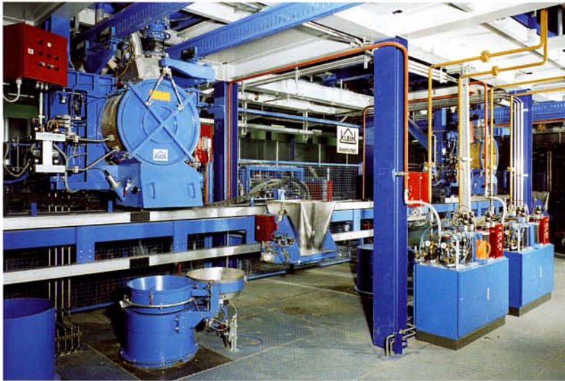
STATORMIX 122 with dosing equipment and distribution vehicle
