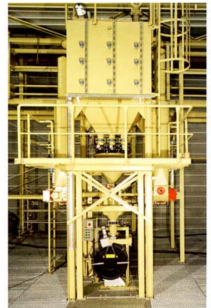
STATORMIX 123 with sand and additive balance
