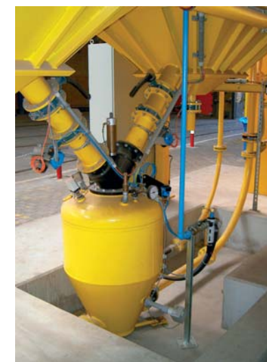
Pneumatic conveyor to supply sand to the individual sand dispensing stations. Gentle conveying process, low consumption of compressed air.
